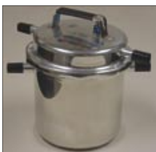
FIGURE 17. Autoclave: high-pressure, saturated steam sterilization
